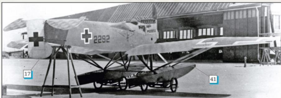
Ordered in April 1918, 2292 was the 5th W.29 completed to C2MGHFT specifications and is pictured here at Warnemünde undergoing acceptance testing. Note the adjustable mount for the wireless generator, early tailplane, black floats and struts, Niendorf propeller and the position of the wing balkenkreuz.
