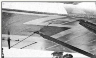
Wing strut attachment detail from W.29 2512 showing aileron control horn and cable exit details. The rib tapes visible here appear to be a very different colour from the rest of the clear doped linen, and while they are possibly a different shade of linen, this effect is mainly due to the matt finish of the rib tapes not reflecting background light as well as the gloss doped wing surface.
