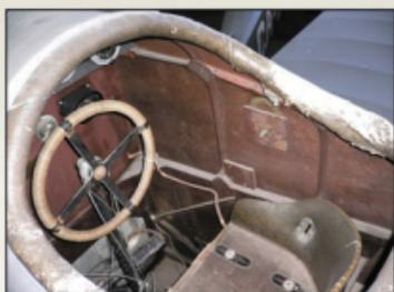
Cockpit detail from IVL A.22 (post war version of the W.29 successor, the W.33, built in Finland). While many details differ from our W.29, this is the only surviving Hansa-Brandenburg monoplane anywhere and therefore provides some useful information for the modeller. This aircraft is located in the Finnish Aviation Museum, Helsinki, Finland.
