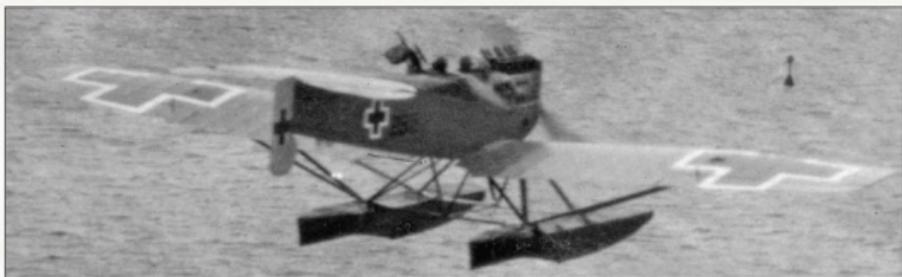
13 W.29 2577 (the full number is not legible) of 1 C Staffell Seeflugstation Zebbrugge displaying the usual location of the wing balkenkruetz, slightly outboard of where they are on 2206. The early production tailplane is evident as are the black painted floats and struts.
