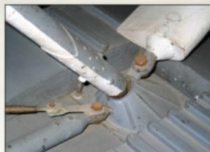
Port float front strut attachment detail.
