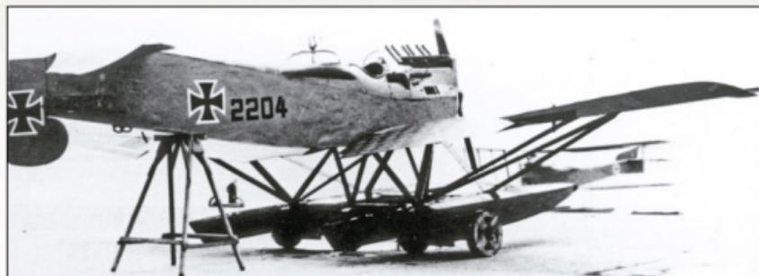
W.29 2204 first flew in March 1918 and went through several refinements before arriving at the final configuration seen here. W.29 2204 was a C3MG aircraft armed with 3 machine guns and no wireless equipment, it is fitted with an Axial propeller here but at other time different propellers were fitted as seen on page 8. Note the style of beaching trolleys and rear fuselage support (13).
